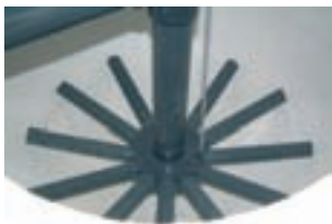
Collector arms detail
